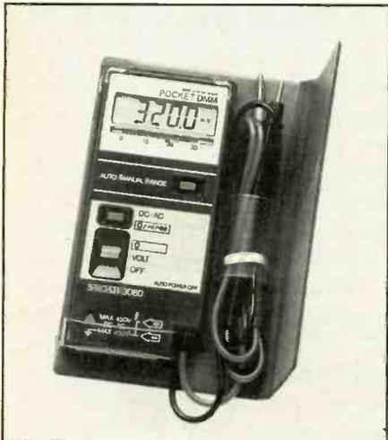
allows the user to select between dc/ac volts and resistance/continuity/junction test. A three-position slide switch applies power in the volts or resistance function and disables power manually. An automatic-off function disables power 10 minutes after the last function/test has been performed to conserve battery power. Power is supplied by two readily available button cells for approximately 250 hours. \$59.95.
