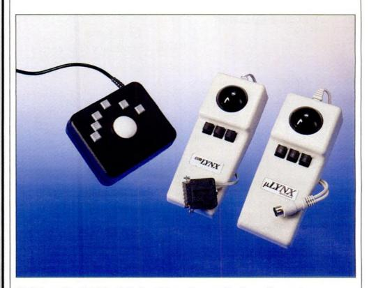
The Fulcrum Trackball Plus (left), from Fulcrum Computer Products, offers precise cursor control and the ability to emulate a wide variety of mice and digitizing pads. The comLYNX (center) and microLYNX (right), from Honeywell Information Systems, emulate the Microsoft Mouse but do not work with Windows.
