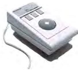
Abaton's **ProPoint** has two buttons on the lower left of the casing. Their significantly different size and shape make it easy to remember which button is which. It's fairly easy for right-handed users to comfortably press both the large click button and the small lock button with their thumb; left-handed people may have to take their fingers off the ball to press
