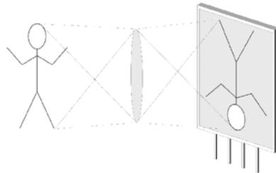
*Fig. 1: Principle of image projection*
