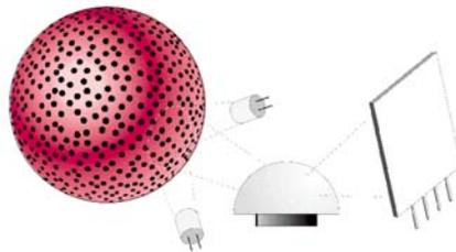
*Fig. 2: TrackMan Marble Wheel optical configuration*
