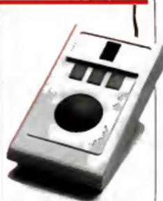
with the trackwheel. The left button is Pick, the right is Enter, and the trackball controls the pointer position.
