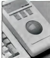
The MicroSpeed PC-Trac features adjustable tracking sensitivity.
