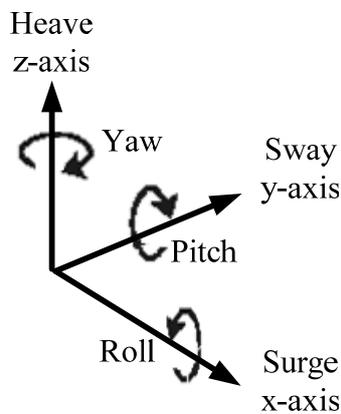
FIG 1. The modes of ship motion
