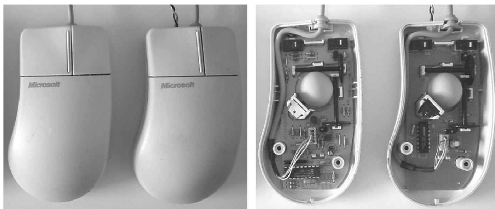
Figure 1. Comparison of the internals of two apparently identical mice: Model MS2.0A, serial interface (left, Mouse 2; right, Mouse 1). The right mouse shows far more chip integration, with a vast reduction in component count.
